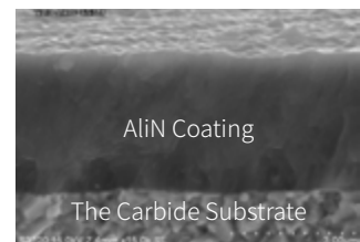
SEM Photograph of Coating
