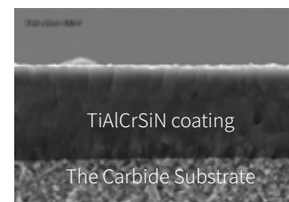
SEM Photograph of Coating
